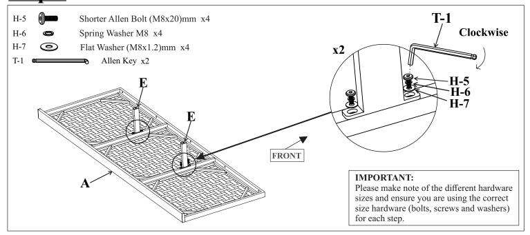
Using a second person to assist you, Place Seat Frame (A) upside down onto a padded, non-marring surface. Position the Center Legs (E) onto the crossbars as shown. Secure both Center Legs (E) to the **Seat Frame (A) with Shorter Allen Bolts (H-5)**, Spring Washers (H-6) and Flat Washers (H-7) using the provided Allen Key (T-1), stacking the hardware in the order as shown. Engage all bolts first, then fully tighten. DO NOT OVER TIGHTEN.
